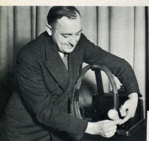
THE INDUCTOTHERM, by creating a magnetic field around its coils, can force current through a man's arm to light a lamp. The device is used in hospitals to induce artificial fever.
